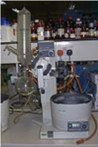
A rotary evaporator is able to distill solvents more quickly at lower temperatures through the use of a vacuum .
